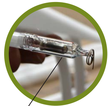
Electrode welded to the end of the tube.
