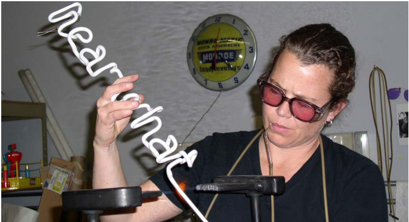
Photo courtesy of PetersonNeon.com. Shawna Peterson demonstrating tube-bending.
