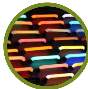
Phosphor-coated glass tubes have a softer glow.
